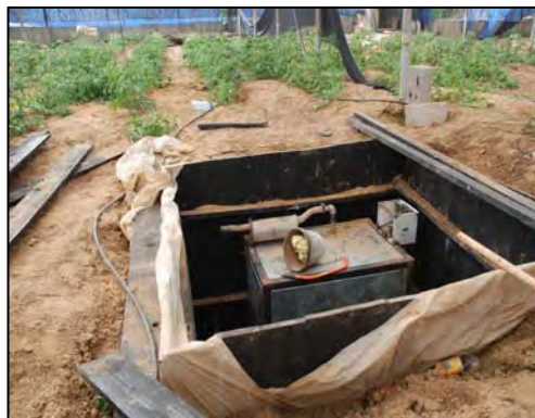
Generator and digging equipment found near a tunnel shaft. The generator was sunk into the ground inside a hothouse to conceal its noise and make it harder to find (IDF Spokesman's website, August 16, 2007).
