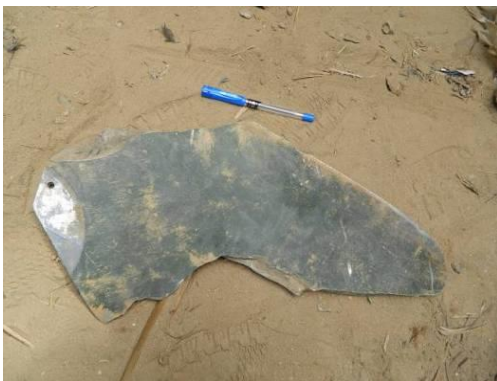
Figure 49.A.2 Rear fin from PAVEWAY terminal guidance unit 216
