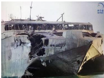
Figure 13.4 Exit point of ASM Port Midships
