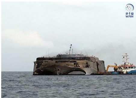
Figure 13.4 Exit point of ASM Port Midships
