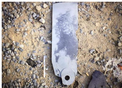
Figure 49.C.3 Probable GBU-12 PAVEWAY II guidance unit rear wing 264
